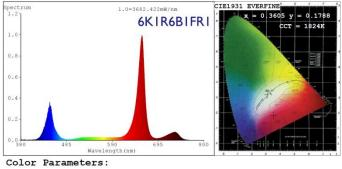
CCT=1961K(Duv=-0.1189) Dominant WL:Ld =-548.3nm Purity=42.0% Ratio:R=48.0% G=45.2% B=6.8% Peak WL:Lp=661.2nm FWHM=20.3nm Render Index:Ra=21.3 AvgR=17.4 R2 =0 R3 =62 R4 =28 R1 = 0R5 = 0R6 =0 R7 = 80R14=86 R8 =0 R9 =0 R10=0 R11=4 R12=0 R13=0 R15=0 Photo Parameters: 1202µmol/s 510W
